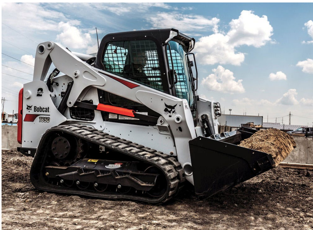
Figure 9. Typical track-mounted skid steer for boring access.
