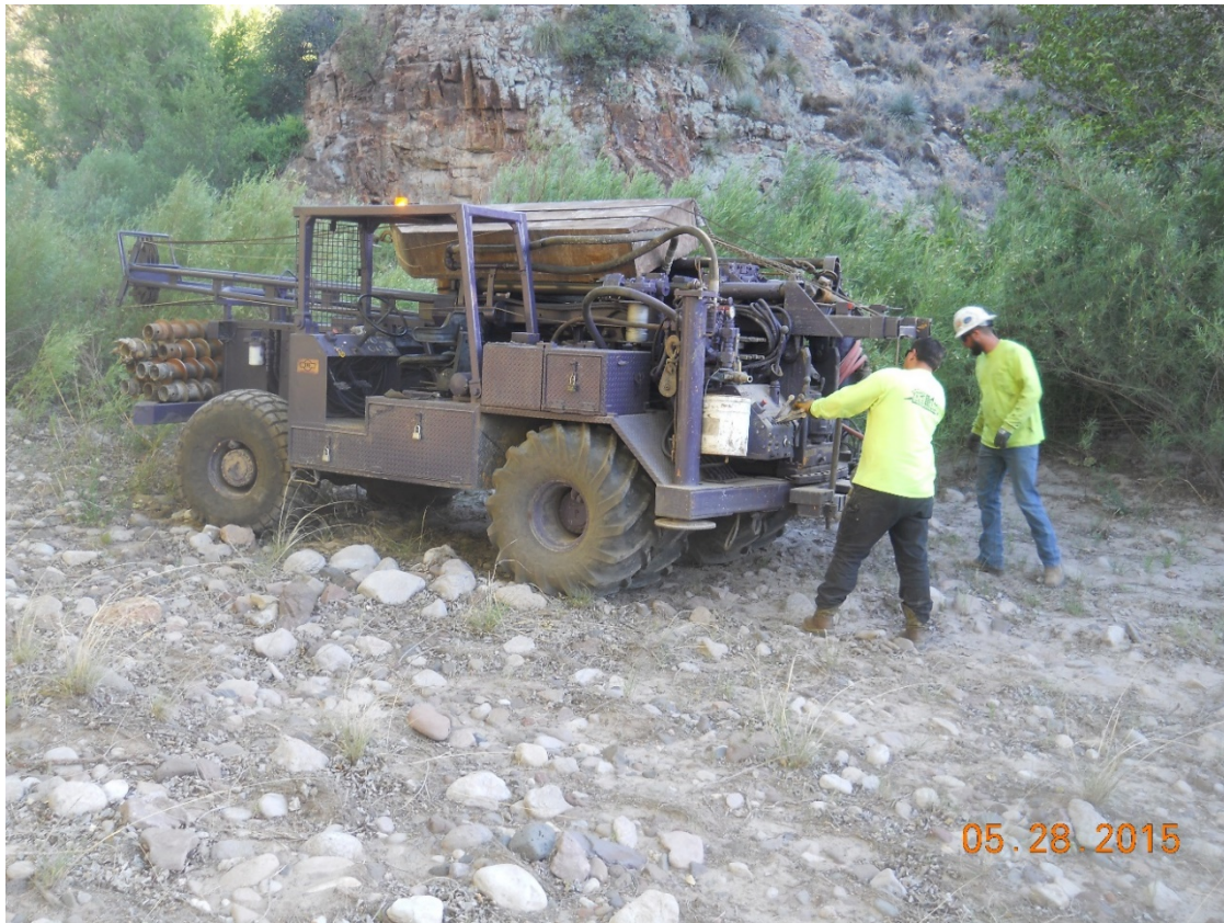
Figure 7. Buggy-mounted drill rig.
